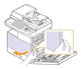
4 Pull the waste toner container out of the machine using its handle.
